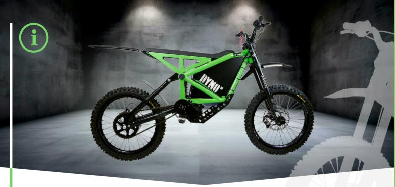
FRAME Aluminium, hand welded
